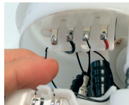
Fig. 3: Typical damage symptoms: the sender unit's cable is detached and the electrical contacts are bent.
