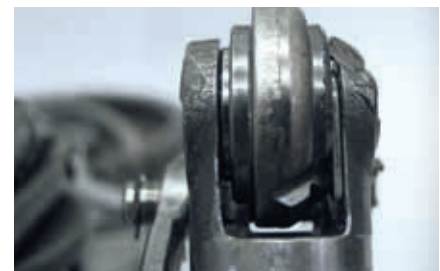
Damage symptoms: cam roller worn on one side
