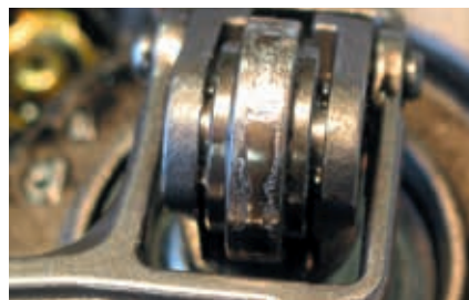
Damage symptoms: Cam roller with pittings due to worn cam.
