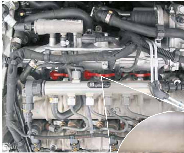
Lever arrangement at the intake manifold in the Opel Vectra (top emphasised in red and detailed view)
