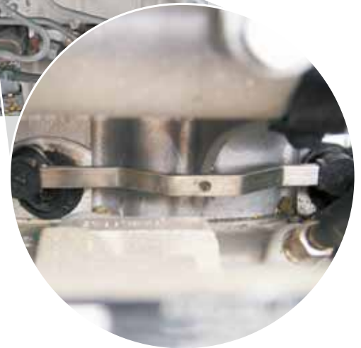
Lever arrangement at the intake manifold in the Opel Vectra (top emphasised in red and detailed view)
