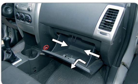
(EN) Open compartment, the filter is placed behind the back wall of compartment
