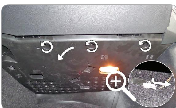
(EN) Loosen the screws and remove the upholstery panel. Disconnect the electric circuit
