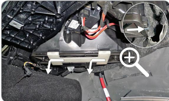
**EN** Remove the protecting device. Move sideways the locks, which hold the cover of the filter chamber
