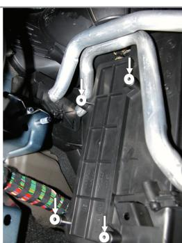
(EN) Loosen the screws and remove the cover of the filter
