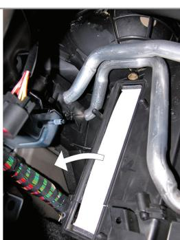
(EN) Gently remove the old filter, put in the new one and carry out the opposite to all the previously mentioned operations in the reversed order
