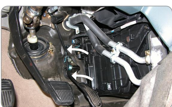
**(EN)** Detach the cover of the filter chamber
