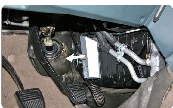
**Carefully remove the first filter, the second one will slide downwards.**
