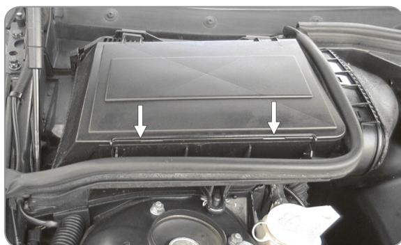
**EN** Undo the latch and open the filter cover
