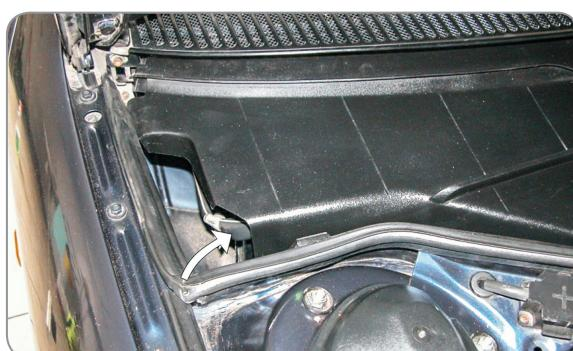
(EN) Remove the rubber seal
