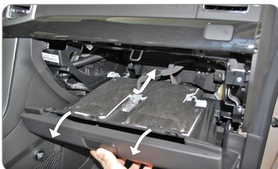
**EN** Disconnect the electric circuit and remove the glove compartment
