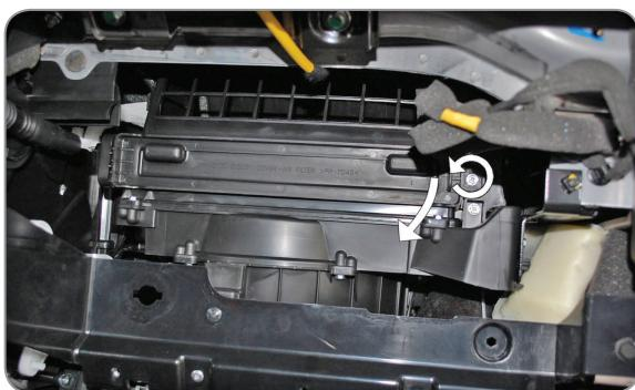
**EN** Loosen the screw on the filter housing, detach the cover of the filter chamber
