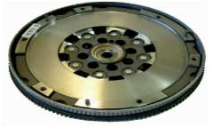
Depth from the clutch bolting surface is 7.9mm. This design was factory fitted ->3/2004.
