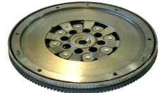
Depth from the clutch bolting surface is 11.9mm. This design was used 3/2004-> but may be retro-fitted to older models.
