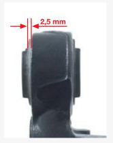
The slot in the new rubber mount must be aligned with the marking on the trailing arm.
