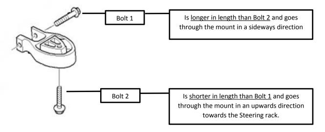
The two bolts securing the lower gear box mounting are noticeably different in length. Please pay extra attention when re-installing the bolts, as <u>failure to insert the correct bolt in the correct location</u> <u>will result in irreparable cast damage to the steering rack</u>. This damage will invalidate the warranty. (please see Fig 2 below).
