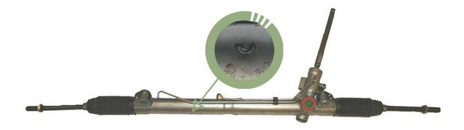
\*\*Please note this type of cast damage will result in a Surcharge Rejection\*\*
