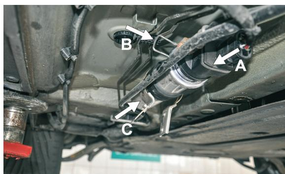
**(EN)** Install pressure regulator (A) with safety device (B) and fuel hose on opposite side of filter (C)
