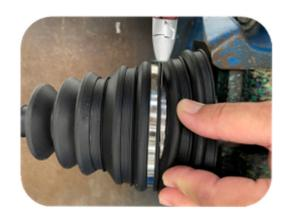
When fitting the universal boot onto the CV-Joint, it is recommended to cut the boot to size after having tightened the clamp.
