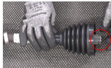
Safety ring set up on the shaft
