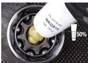
Half quantity in the joint
