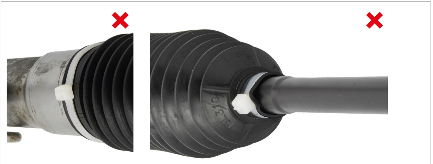
Fig. 7: Bypass: Defective seal with cable ties
