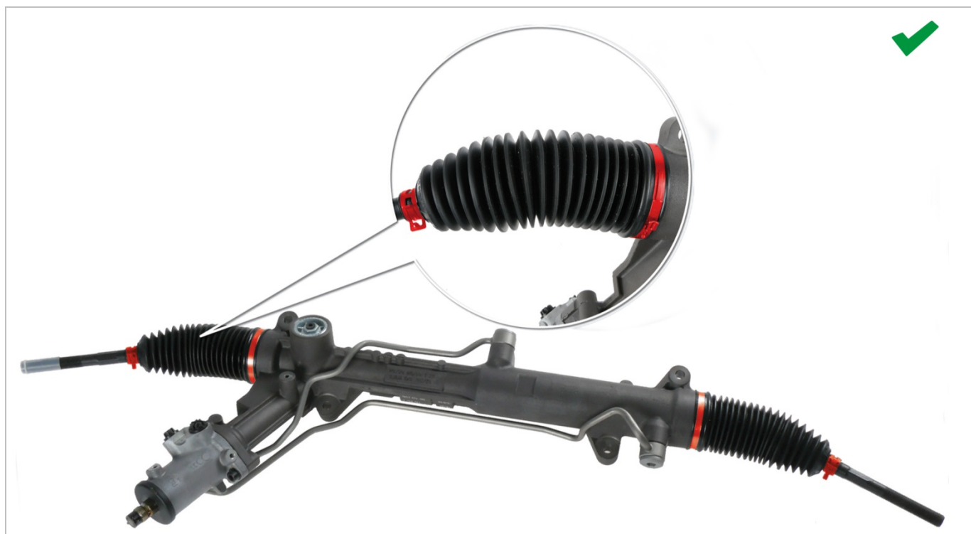
Fig. 1: Steering gear with hydraulic power steering: Correctly assembled steering boots
