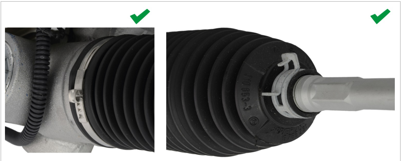
Fig. 5: No bypass: Correct seal with metal clamp
