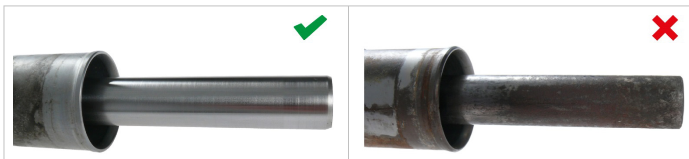
Fig. 2: Steering rack without corrosion
