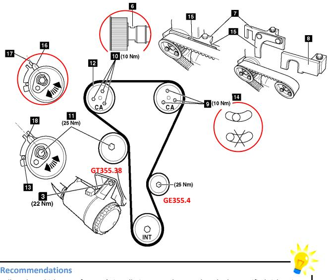
Follow the vehicle manufacturer's installation procedures and apply the specified tightening torques.
