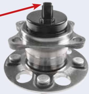
**GB** The ABS sensor connector pins in this rear wheel bearing are relatively thin and delicate.
