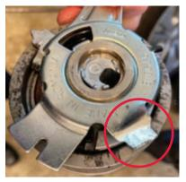
**Tensioner failure tab damage** Cause: incorrect setup procedure
