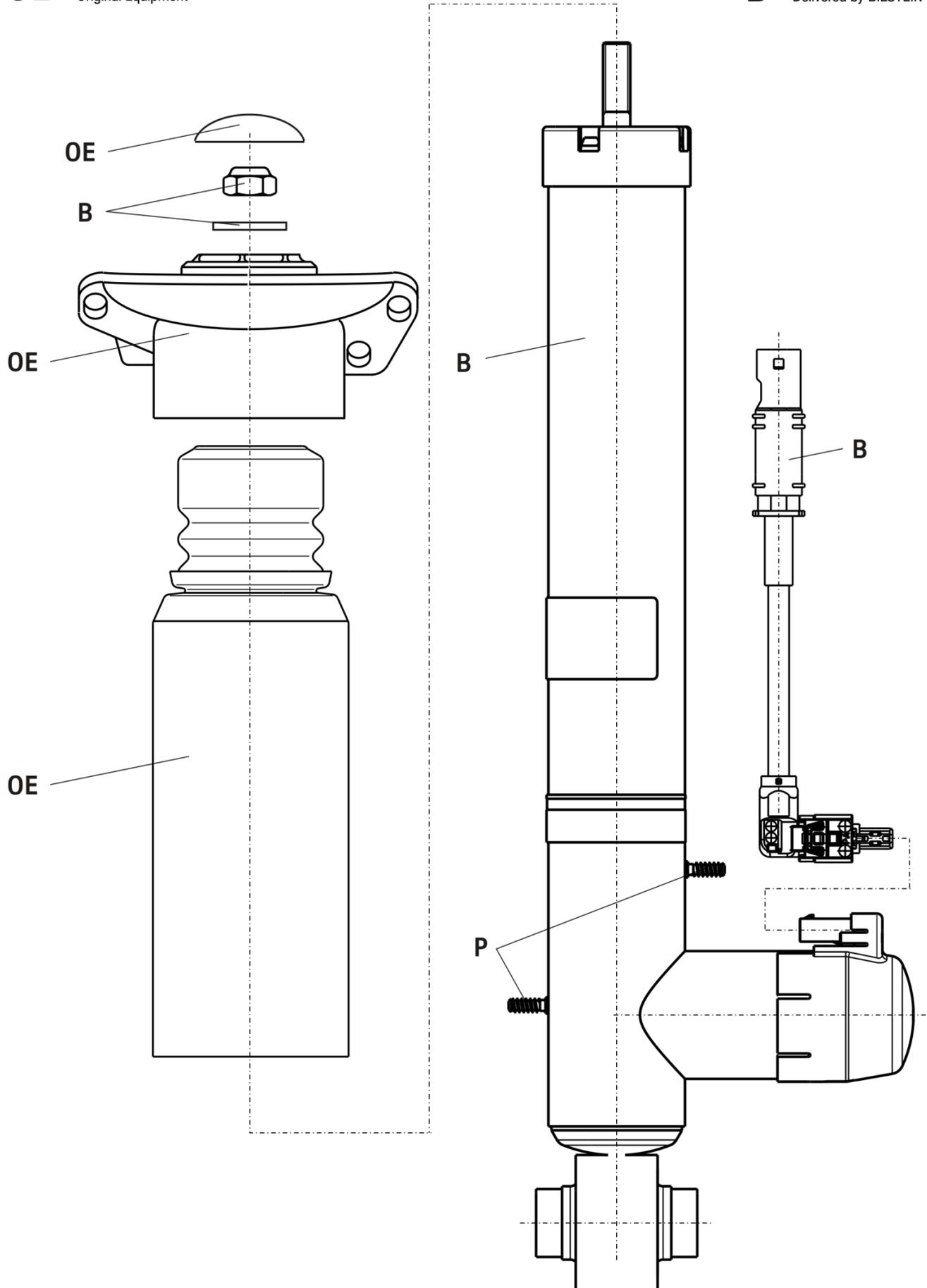
**Hinterachs- Höhenverstellung - adjustment assembly for rear axle**
