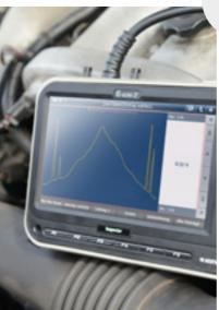
the throttle valve actuation. That's how plausible signal outliers can be located. Note: Alternatively the inspection can be performed as a so called quick check with the Inspector's oscilloscope.
