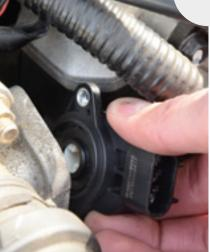
7. Last but not least, the new sensor's function is checked and the relevant entry in the fault memory is deleted. All done!
