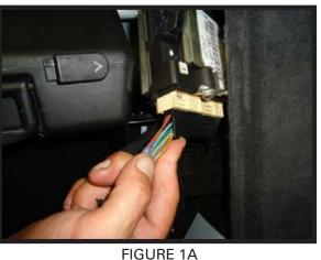
2. REMOVE BOTH PLUGS LOCATED ON THE CONTROL MODULE. (FIGURE 1B)
