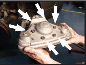
FIGURE 10-5 10. REMOVE THE AIR STRUT FROM THE UPPER MOUNT. (FIGURE 10-6)
