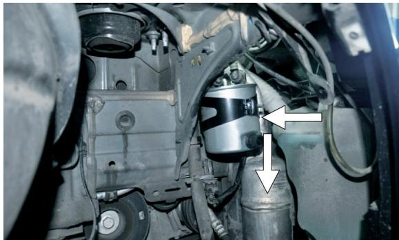
**(EN)** Install fuel heater valve element, fuel hoses and place filter in seat
