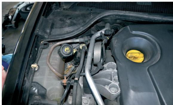
**(EN)** Pump with manual pump till resistance is felt, start the engine, check for leakage
