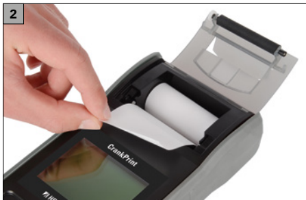
Fig. 2 Inserting the roll of paper
