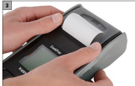
Fig. 3 Closing the cover of the paper compartment
