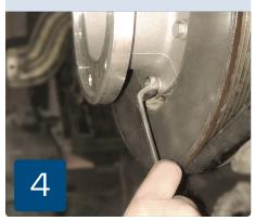
Introduce the fan clutch wheel into the gap between the radiator and the engine.
