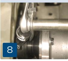
Connect the fan clutch connector to the vehicle connector.
