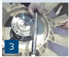
Install the aluminium adapter on the vehicle. Use the 6 M8x30 screws provided. Tighten at a tightening torque of 30Nm.
