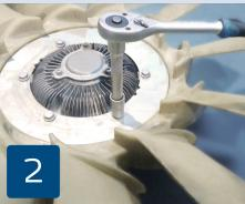
Install the fan wheel on fan clutch using the 6 M8 screws provided. Tightening torque 25Nm. On fan clutch, the fan wheel is installed on the rear part of the aluminum chassis.
