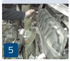
With the fan clutch wheel moved towards the radiator, assemble the fan ring passing it through the gap between the aluminum adapter and the clutch.
