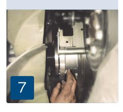
Install the fastening flange of the cable by tightening the M8 screw of the vehicle.
