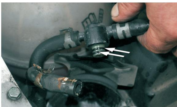
(EN) Install new sealing rings onto regulation valve element
