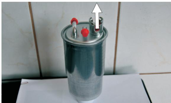
**(EN)** Remove the safety plug and fill new filter with clean diesel oil
