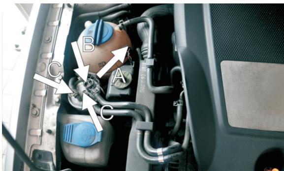
(EN) Remove the fastening clamp (A) and regulating valve (B), loosen the fuel hose bands, remove hoses (C)
