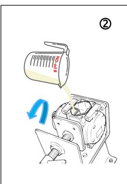
Flush the ND-oil 6 out, by pouring ND-oil 8 in the suction port (LP) and rotate the compressor by hand.
