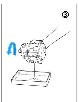
Make sure that all ND-oil 6 is removed and only ND-oil 8 is visible.
