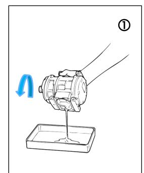
Drain the ND-oil 6 by keeping the compressor upside down and rotate the compressor shaft by hand.
