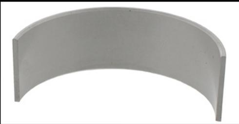
The upper half is recognised as the thrust side as during the combustion cycle, it is subject to the highest load. The composition of the upper half big end bearing can vary, most widely used is LC/LCX, a heavy duty specification. The colour of the upper shell is usually a matte white/grey.
