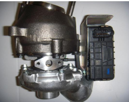
Once mounted on the vehicle, the turbo may not function correctly. This is because the ECU or DDE needs to be reprogrammed by the authorised technical service in order to function correctly, given the fact that the position regulator and the diagnostics are both incorporated in the servomotor.
