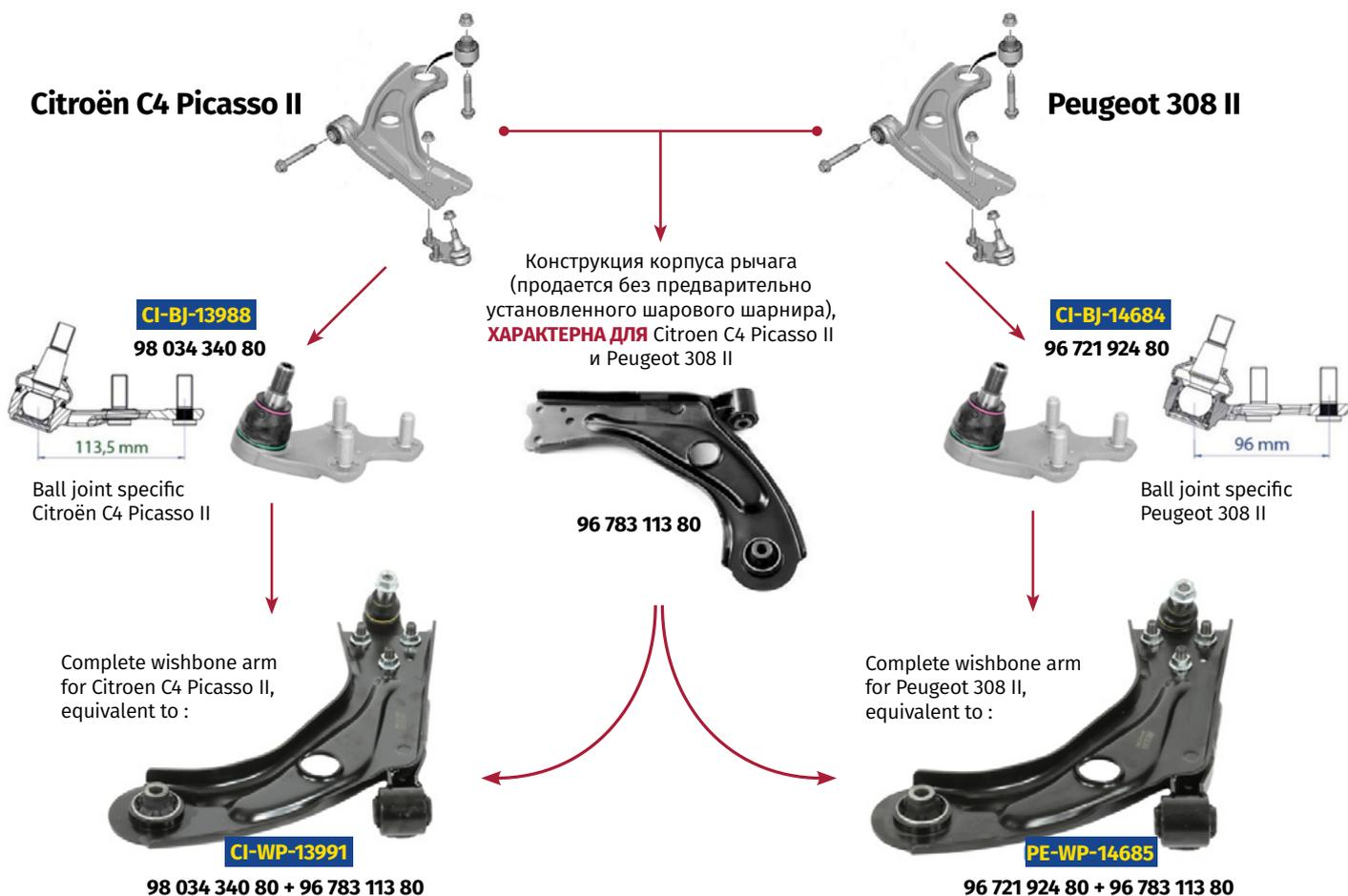
⚠ **When ordering MOOG parts, from an OE equivalent, check the application of the reference**
