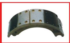
MAIN • Lining radius is larger than actual drum diameter **REASONS** • Bedding-in period for the lining was too short
