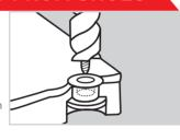
If a service tool is not available, the clenched head of the rivet may be removed by drilling or chiselling. (Extreme care must be taken to ensure the brake shoe rivet holes are not damaged during this operation).
