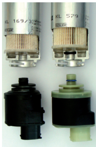
Figure 2: The matching filter for each respective inline fuel filter
