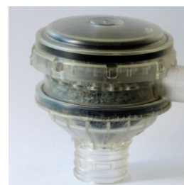
Crankcase ventilation system with oil mist separator
