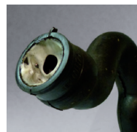
Crankcase ventilation: clogged by an emulsion consisting of condensate and engine oil
