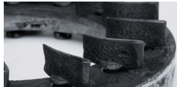
VTG: heavy oil carbon build-up blocking the mechanism
