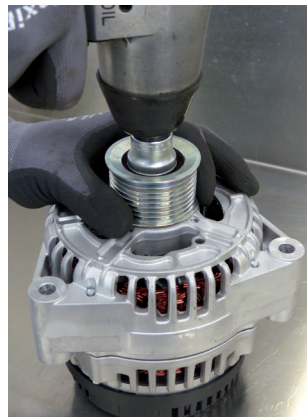
Figure 2: Impact drivers are only used to loosen the pulley, NEVER to tighten it!
