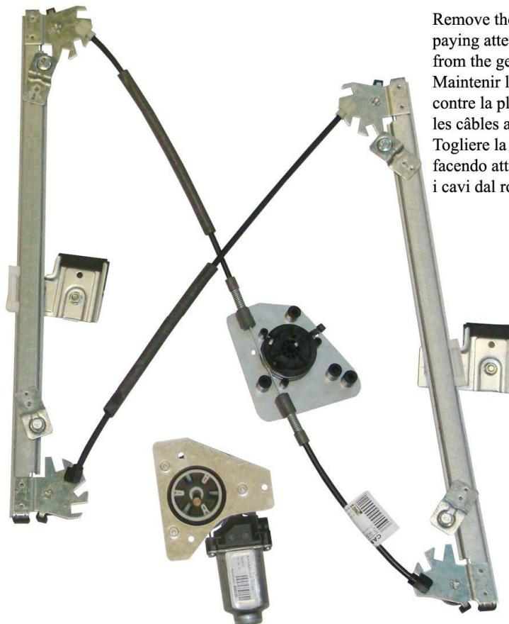
Remove the gear pvc clamp, paying attention not to unroll the cables from the gear.
