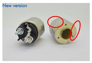
The most visible change (red circles) is the double facet on the body in order to get easy the placement on the specific starter bracket.
