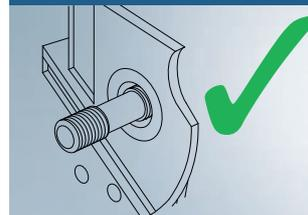
Studs (6 and 10) screwed in all the way to the stop
