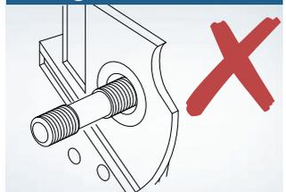
Studs (6 and 10) not screwed in all the way to the stop
