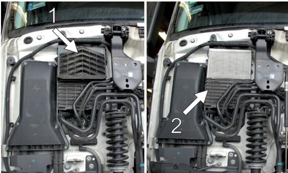
**(EN)** Remove the filter housing
