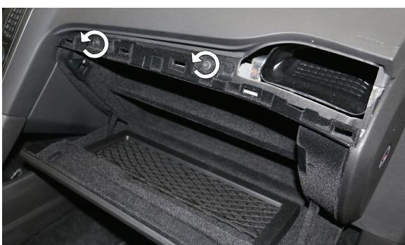
(EN) Loosen the screws on the glove compartment
