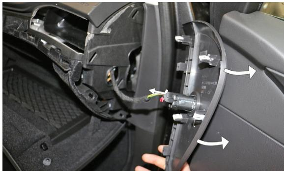
**(EN)** Remove the upholstery panel, disconnect the electric circuit
