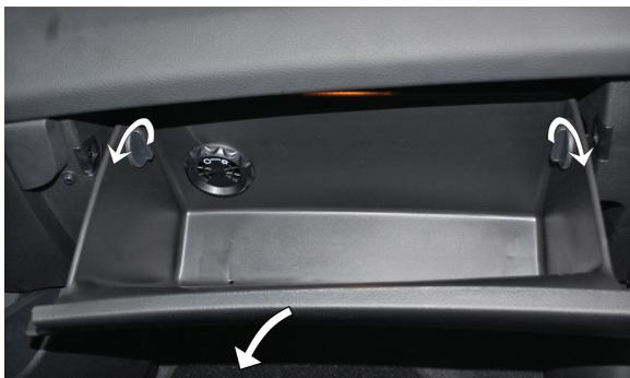
(EN) Open the glove compartment, unclasp the compartment, remove the glove compartment
