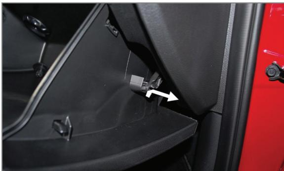
EN Remove the protecting device.
