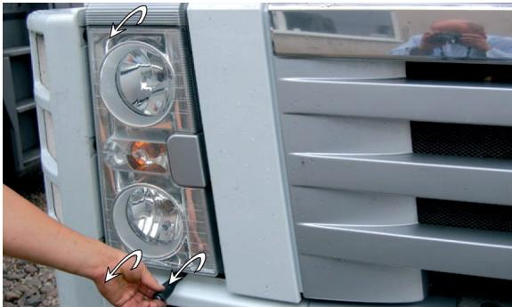
(EN) Slightly lift the car cabin, unscrew the screws fastening the light
