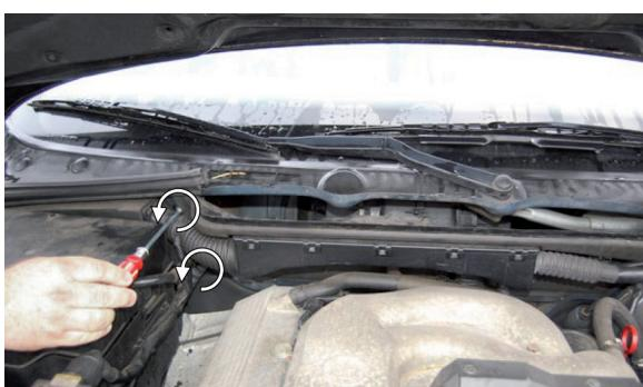
(EN) Unscrew the screws fastening the element shown on the picture
