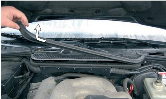
(EN) Remove the rubber seal
