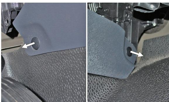
(EN) Remove the protecting device
