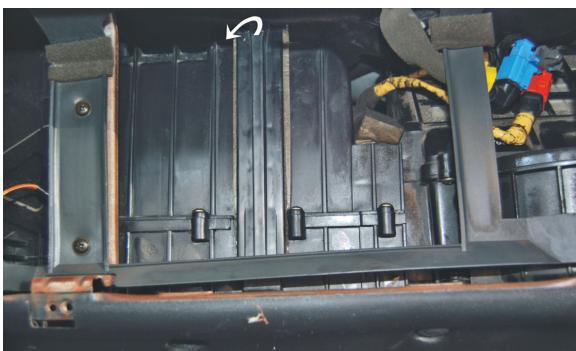
(EN) Remove the cover of the filter chamber
