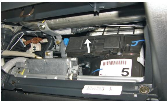
(EN) Detach the cover of the filters chamber
