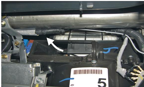
**(EN)** Take out the old filter from the socket, put in the new one, close the cover, secure it with the latch and repeat the operation for the other filter
