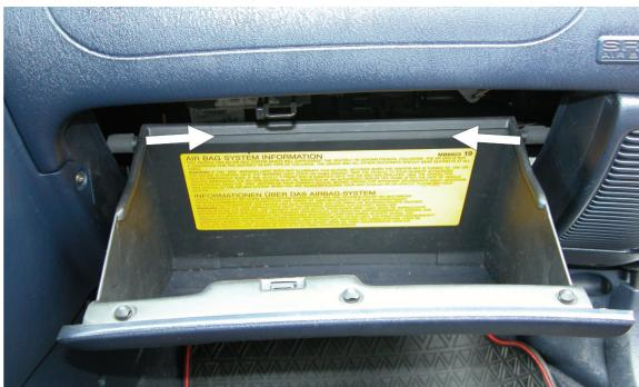
(EN) Remove the glove compartment
