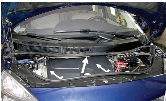
(EN) Remove the engine housing
